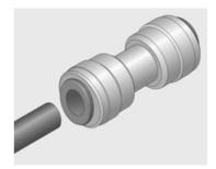
Step 1. Cut the part of the tube to be inserted into the fitting to plane the end. Make sure to use a clean tube without any foreign material or cracks.
